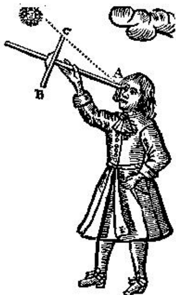
Figure 3. Using a cross-staff to measure angles
