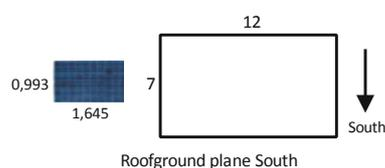
cm from the others, in order to create enough space for the technician to be able to repair the system in case of damage or break down. For maximum efficacy in the production of electric current the panels should have south exposure, while their inclination angle is suggested to be  $30^{\circ}$  from the horizontal. According to existing regulations, the panels should be 1m from the perimeter line for safety reasons. Find the maximum number of panels that can be placed on the roof.
